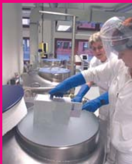
Computer-controlled equipment freezes the cord blood products to -145°C
