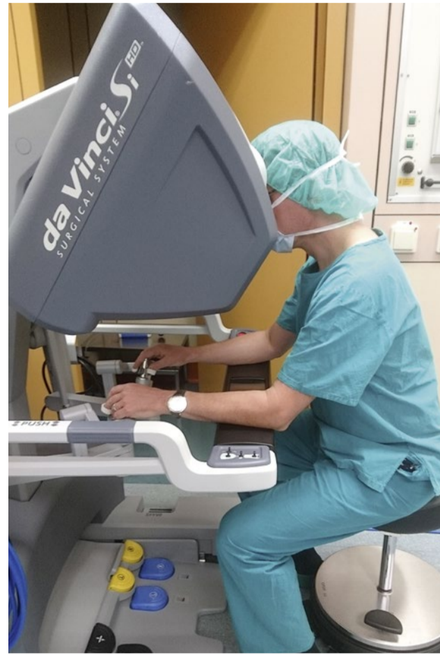
An assistance system for minimally invasive spinal surgery: Robot-assisted positioning of screws on a model of the lumbar vertebrae at the Research Project Centre for Sensor Systems (ZEISS), University of Siegen and Neurosurgery Karlsruhe
